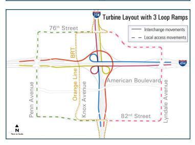
The Turbine interchange concept has been carried forward for additional design. The illustrations above show a turbine concept with one loop and a turbine concept with three loops. The solid lines represent the proposed modifications to the interchange. The major freeway movements would be accommodated via the new interchange and local roadway access would be provided via existing interchange ramps at Penn Avenue, Lyndale Avenue, 82nd Street and 76th Street, shown by the dashed lines.
